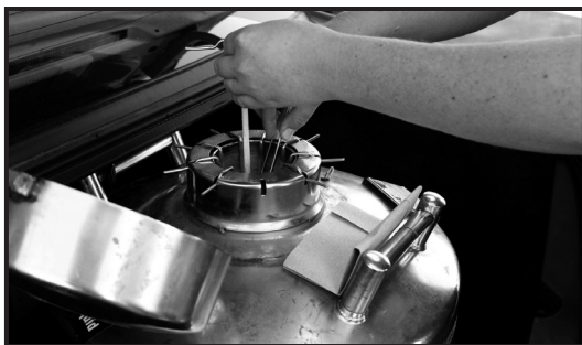
Fig. 1: Raise canister just high enough to grasp the top of the cane with a tweezers – about five inches from top.
